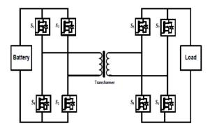
Fig. 1. Isolated DC-DC Converter
