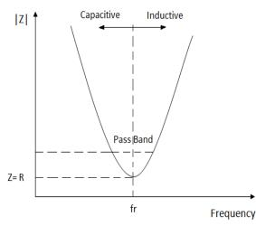
Fig.1. Single Tuned harmonic filter |Z| vs Freq
