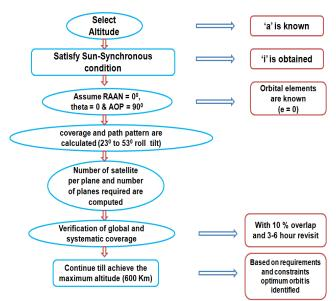
Fig. 3. Structured satellite constellation design procedure
