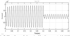
Fig.7. Waveform of phase A of load current (with MCR) FFT analysis after connecting MCR is shown in Fig.8.
