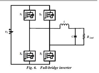
The wave shape of output voltage are square, quasi-square or distorted sinusoidal. Inverters used in low and medium power applications normally give square or quasi-square wave output which is acceptable. However, in high-power applications sinusoidal waveform is required, so inverters are carefully designed to give sinusoidal output with low distortion. Inverters are widely used in industrial and household applications. Fig. 6 shows the full-bridge inverter [9].
