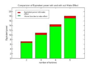
Fig. 5. No. of turbines vs Equivalent power
