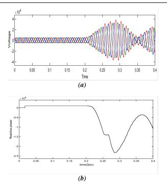
Fig.12. with SVC (a) voltage (b) reactive power
