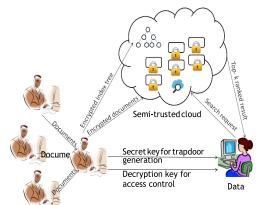
Figure 1: The architecture search over group shared encrypted cloud data
