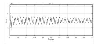
Fig.5. waveform of phase A of load current (without MCR)
