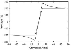
Fig.3. Dynamic V-I characteristic of arc furnace
