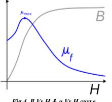
Fig.4. B Vs H & µ Vs H curve
