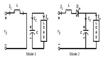
Fig. 4(b) Equivalent circuit of modes of operation
