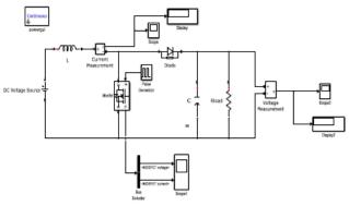
Fig. 9(a) Simulation model of boost converter
