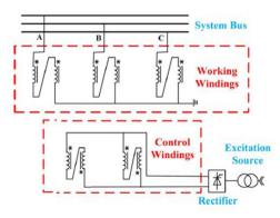
Fig.3. structure of MCR winding
