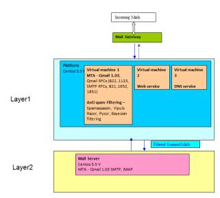
Fig 3. Spam and virus detection using multi layer architecture
