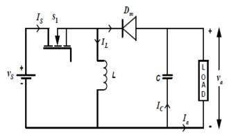
Fig. 5(a) Circuit diagram of buck-boost converter
