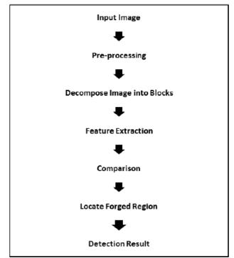
Fig. 5 General Flow of Image Forgery Detection
