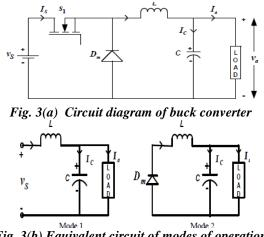
Fig. 3(b) Equivalent circuit of modes of operation
