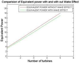
Fig. 6. No. of wind turbine generators vs Equivalent power with and without wake effect
