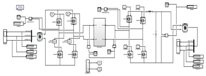
Fig. 11(a) Simulation model of isolated dc-dc converter
