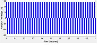
Fig. 11(e) Simulated result of primary voltage of transformer
