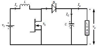
Fig. 4(a) Circuit diagram of boost converter
