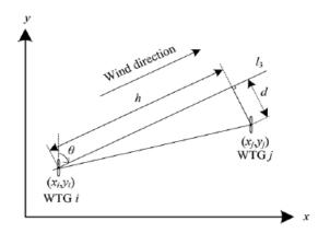
Fig. 3. Horizontal and Deviating distances of two WTGs
