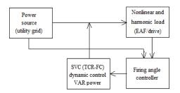
Fig.1. Block diagram of proposed scheme
