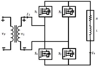
Fig. 7. Single-phase full bridge rectifier
