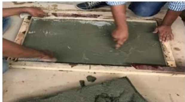
Fig 1 (b): Casting of panel specimens
