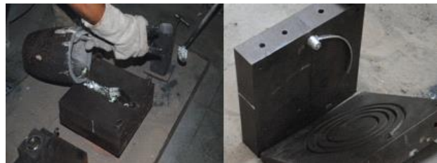
Fig.5 Pouring of molten metal and demoulding of spiral casting
