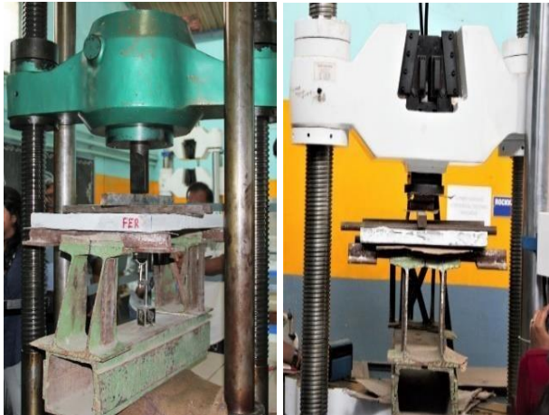
Fig 2: Flexural testing of panels
